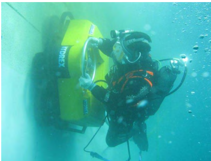
Ecospeed is a Surface Treated Coating intended for regular underwater treatment
