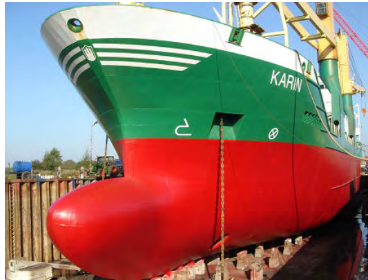
Fresh application of Ecospeed on a general cargo vessel.
