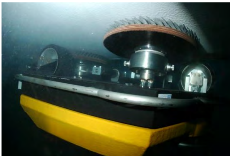
Semi-automatic maintenance tool in use for the underwater treatment of Ecospeed on large areas.
