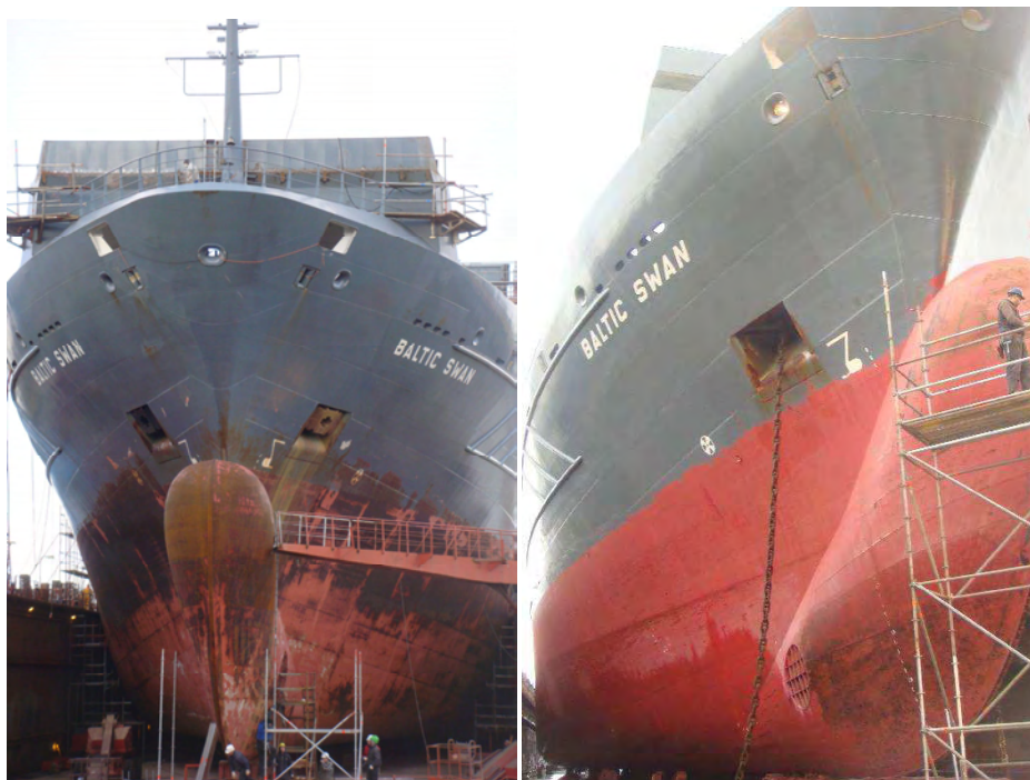
Comparison of the same container ship with a conventional biocidal antifouling (left) and Ecospeed (right) after spending subsequent periods of 2.5 years operating in the Baltic Sea.
