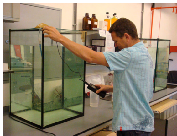
Effluent analysis after conditioning Ecospeed
